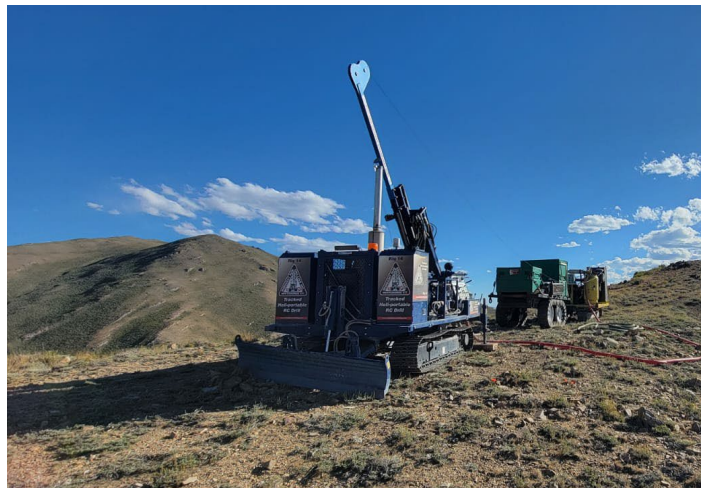
Photo 1 - RC Drill Rig to test Trenton and Philadelphia Copper Prospects
