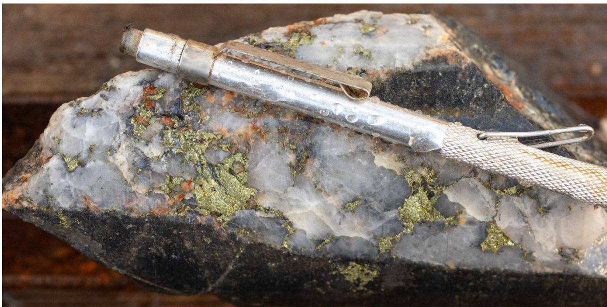
Figure 1. Coarse grained chalcopyrite in quartz veining at down-hole depth of 14m hosted in a 2.7m interval of potassic altered volcanoclastic sediments. Visual estimates of chalcopyrite abundance in this 2.7m interval are between 0.6% and 0.9% by volume, representing indicative copper grades between 0.2% and 0.3% Cu.
