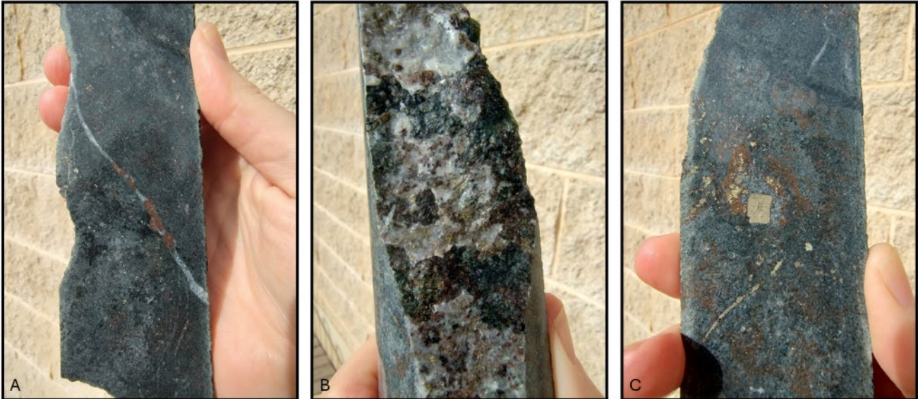
Figure 4. Photos of drill core from drillhole BUDD100, from left to right (A) disseminated chalcopyrite and bornite with sphalerite occurring along calcite veins (450.9m). (B) disseminated chalcopyrite and sphalerite (451.1m) and (C) disseminated chalcopyrite, pyrite, and sphalerite with pyrite and chalcopyrite veining (451.2m).
