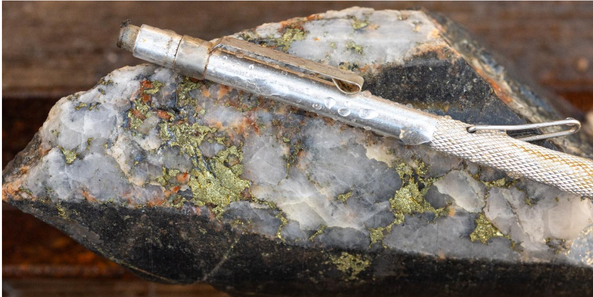
Figure 3 Coarse grained chalcopyrite in quartz veining at down-hole depth of 14m hosted in a 2.7m interval of potassic altered volcanoclastic sediments. Visual estimates of chalcopyrite abundance in this 2.7m interval are between 0.6% and 0.9% by volume, representing indicative copper grades between 0.2% and 0.3% Cu.
