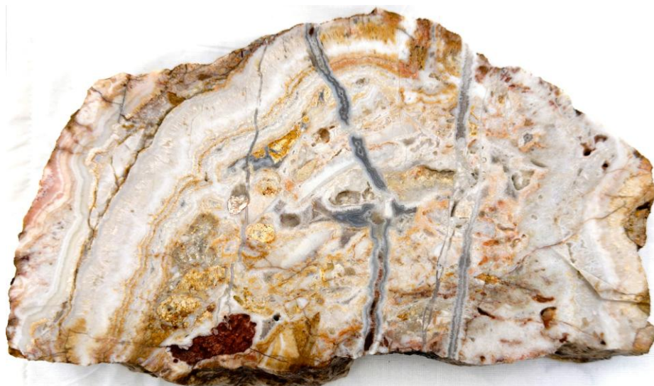
Figure 1: Crustiform-colloform silica-sulphide banded quartz vein in rock chip (sample FC25_007) which assayed 12.45g/t Au, from Francis Creek.
