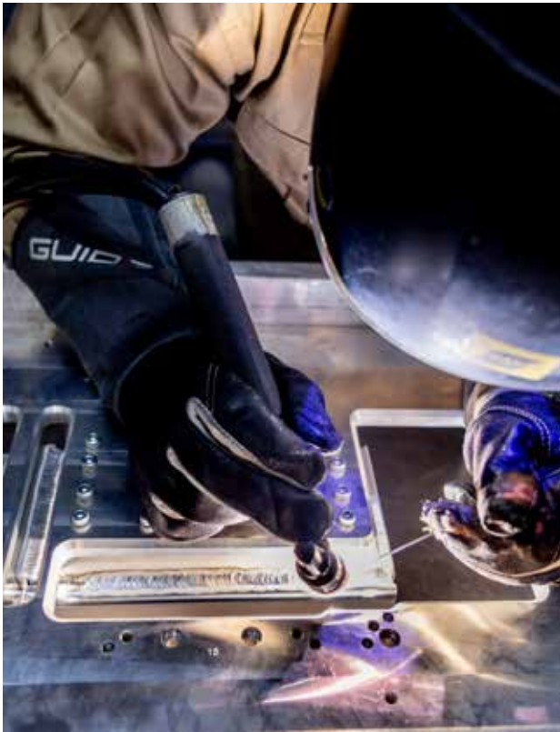
TIG welding in progress on one of PWR’s specialised products
