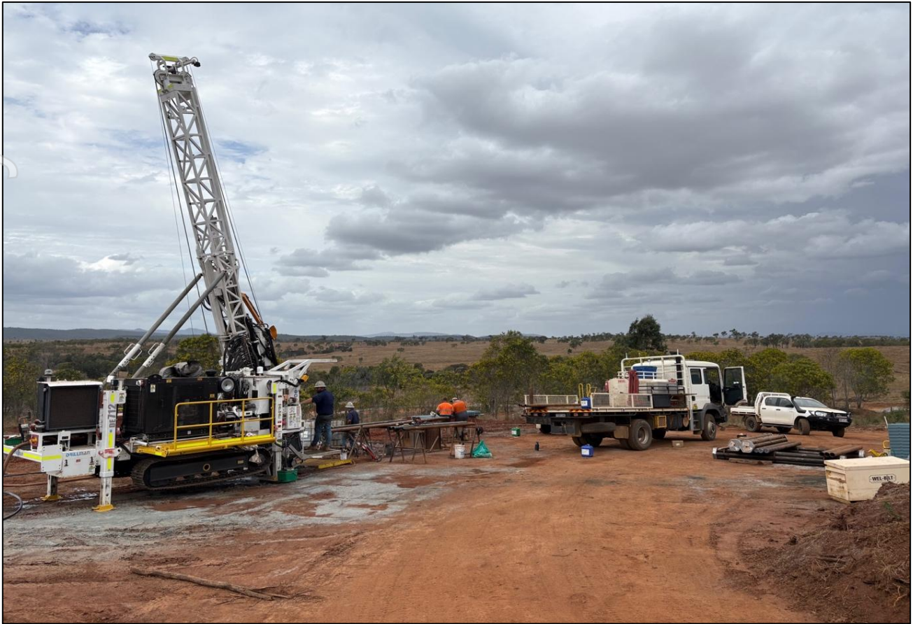
Figure 3: Diamond rig drilling first diamond tail at the Sulphide City deposit.
