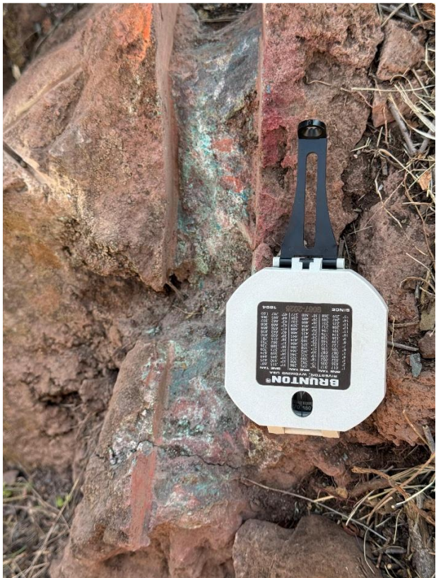
Image 2a & 2b: Diamond saw cut channels with copper mineralisation (green malachite), Gossan 1
