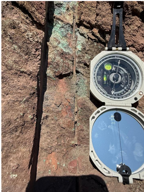
Image 2a & 2b: Diamond saw cut channels with copper mineralisation (green malachite), Gossan 1
