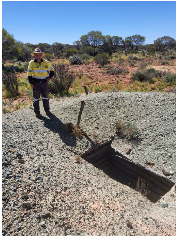
Figure 4. Oaklands Prospect — historical timber-lined shaft and associated costeans along a shear-parallel corridor (MGA94 Z51 - 384520mE 6793165mN)
