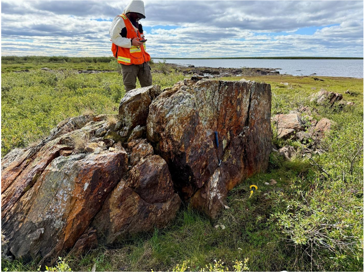
Figure 9: | Spectre- Outcrop of semi-massive to stockwork veined sulphide within a felsic tuff consisting of pyrite -sphalerite-chalcopyrite and the location of sample M209541.
