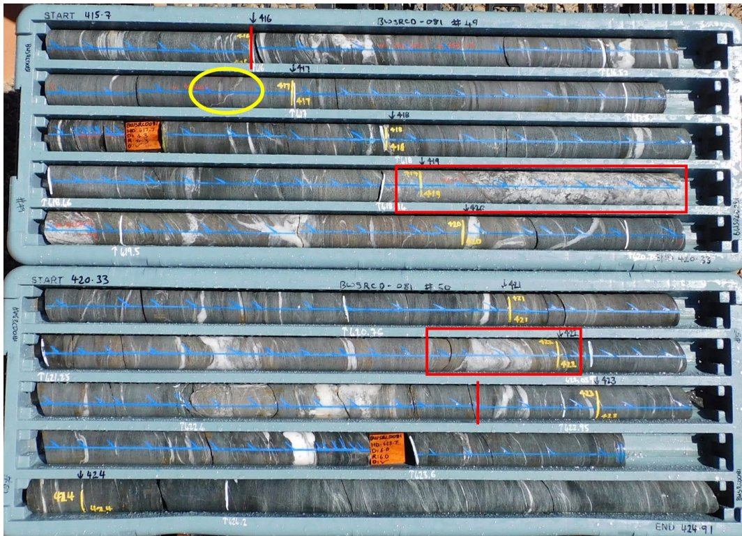
Figure 2. Photo of 6.8m wide alteration zone from 416-422.8m (red markers) with intense quartz carbonate veining intersected in drill hole BWSRCD081. Visible gold bearing vein at 416.8m highlighted by the yellow ellipse, and location of samples shown in figure 3 highlighted by red boxes.
