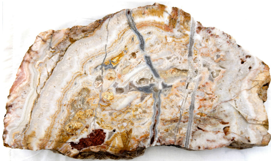
Figure 4: Crustiform-colloform silica-sulphide banded quartz vein in rock chip (sample FC25_007) which assayed 12.45g/t Au, from Francis Creek.
