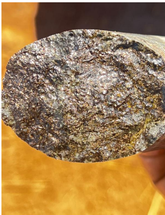
Figure 3: MPYD001 Sulphide alteration/ mineralisation in NQ core at a depth of 85m.
