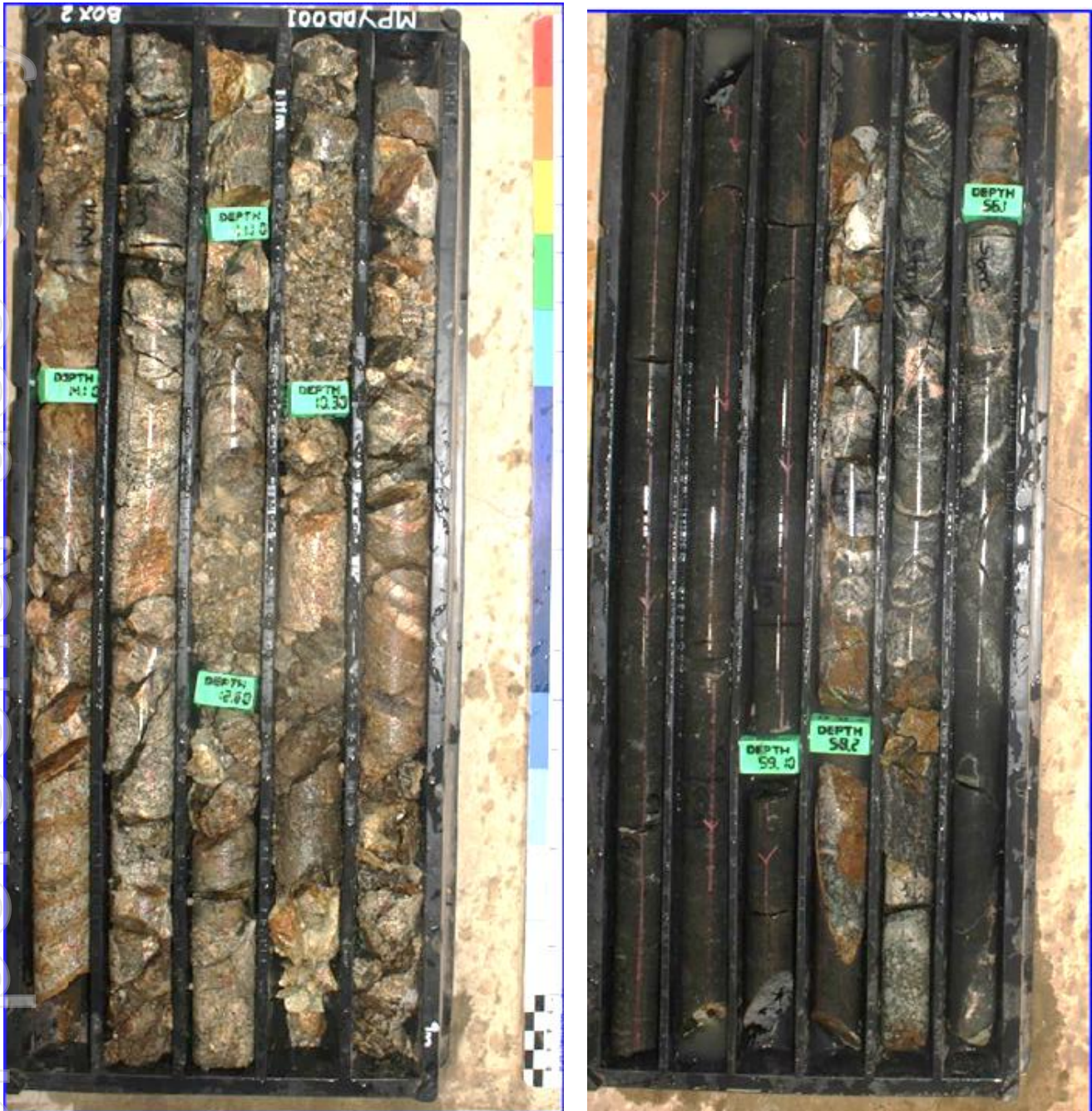
Figure 9 ; Mpyupyu anolmaly drillhole MPYDD001- (Left) Potassic alteration (finitisation) and brecciation of wall rock adjacent intrusive system, Right - Barite rich dyke or stringer at 57 to 58 m down hole indicating increased sulphide activity
