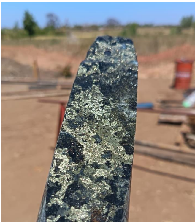
Figure 3: MPYD001 Sulphide alteration/ mineralisation in NQ core at a depth of 85m.
