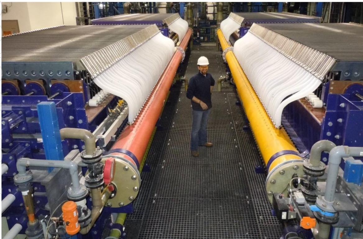
Figure 1: Example of two BICHLOR™ Electrolyzers utilised to produce \text{H}_2 \text{ (g)} + \text{Cl}_2 \text{ (g)} + 2\text{NaOH (aq)}
