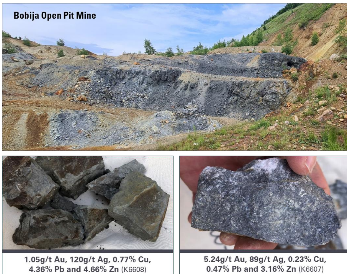
Figure 3: View of Bobija open pit mine with rock chip samples from the massive sulphide zone shown.
