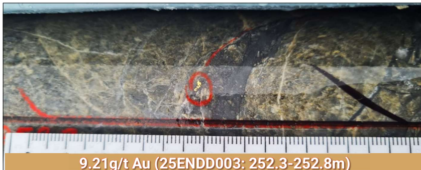
Photo 3. Sample photo of 25ENDD003 from 252.3m – 252.8m @ 9.21g/t Au with visible gold circled in red associated with very fine-grained pyrite-arsenopyrite-arsenian pyrite vein (dark colour).
