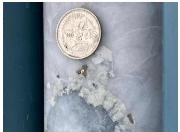
Figure 4 Visible gold at 600.2m depth associated with arsenopyrite in a quartz-carbonate vein
