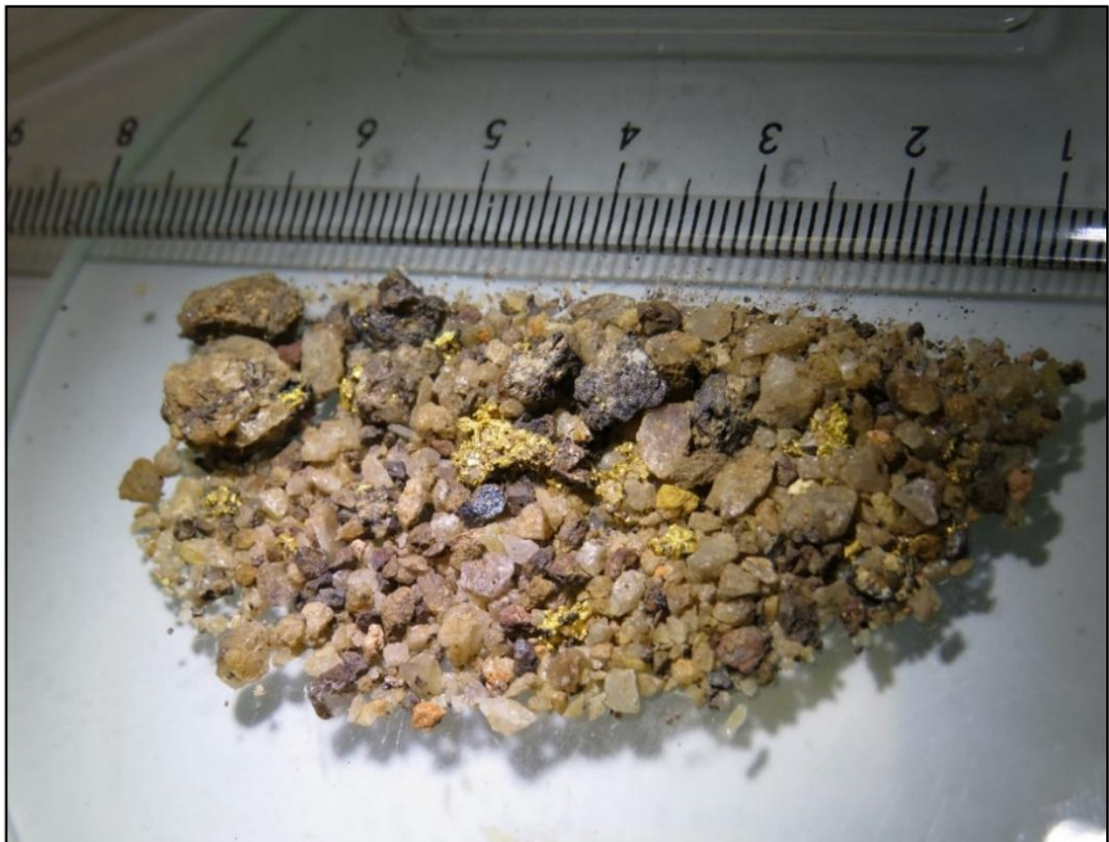
Photo 1: Visible gold within feruginized quartz breccia (drill chips; OGGRC266; 9-10m; ASX Announcement 8 September 2020).
