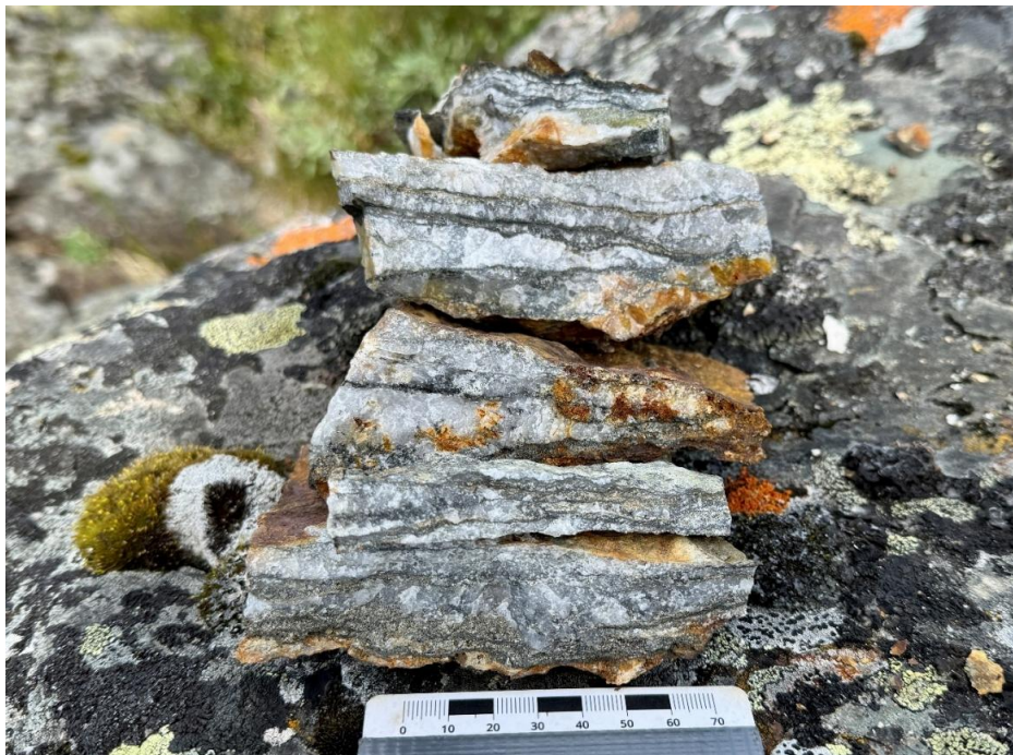
Figure 6: | Quantum Sample M209535. A quartz vein with mm scale laminations of pyrite-arsenopyrite-chalcopyrite-galena.
