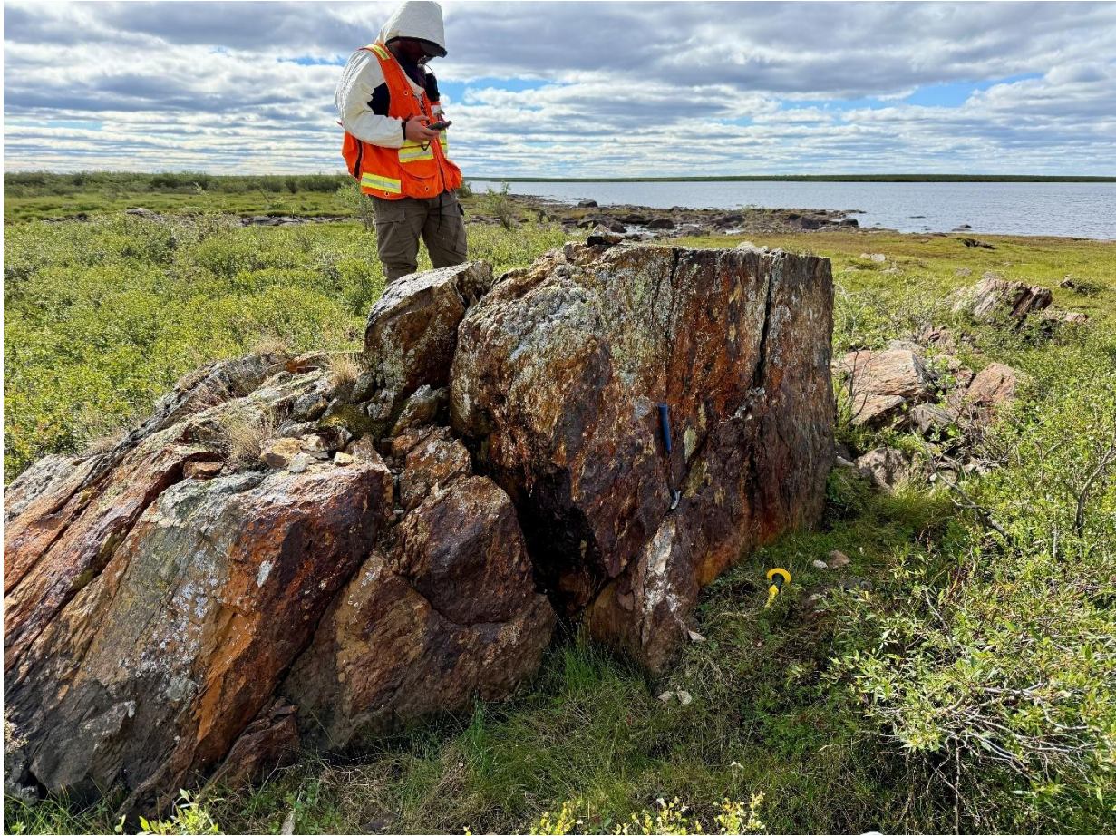
Figure 9: | Spectre- Outcrop of semi-massive to stockwork veined sulphide within a felsic tuff consisting of pyrite -sphalerite-chalcocopyrite and the location of sample M209541.
