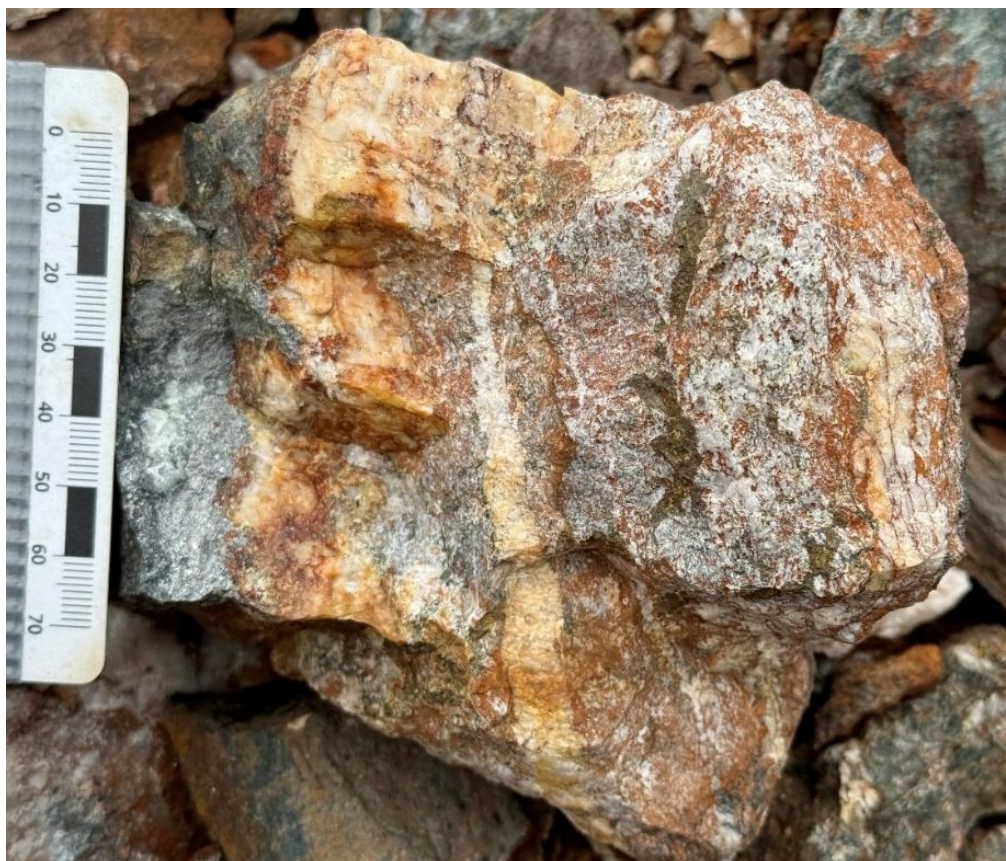
Figure 4: |Jaws Sample M209503 – quartz veined iron carbonate altered mafic volcanic with 2cm band of arsenopyrite from the northeastern extents of the discovery zone.
