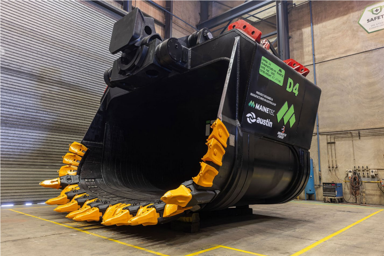
Austin has manufactured the first 4100XPB dipper bucket fitted with Bierwith Forge's GET technology
