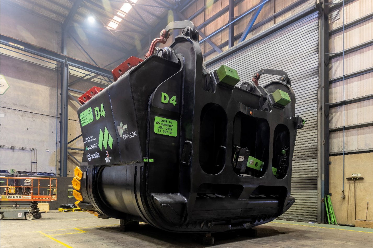
Austin has manufactured the first 4100XPB dipper bucket fitted with Bierwith Forge's GET technology
