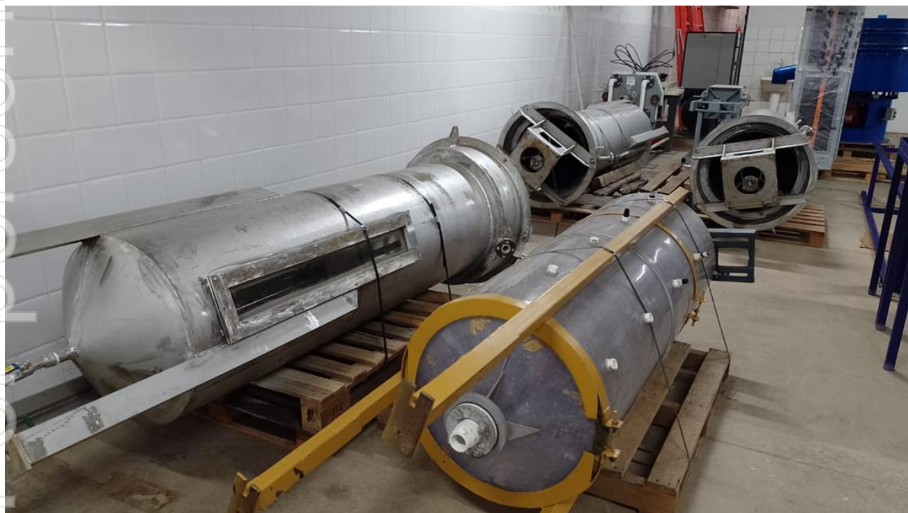
Figure 3: Four CCDs will be used in the Pilot Plant
