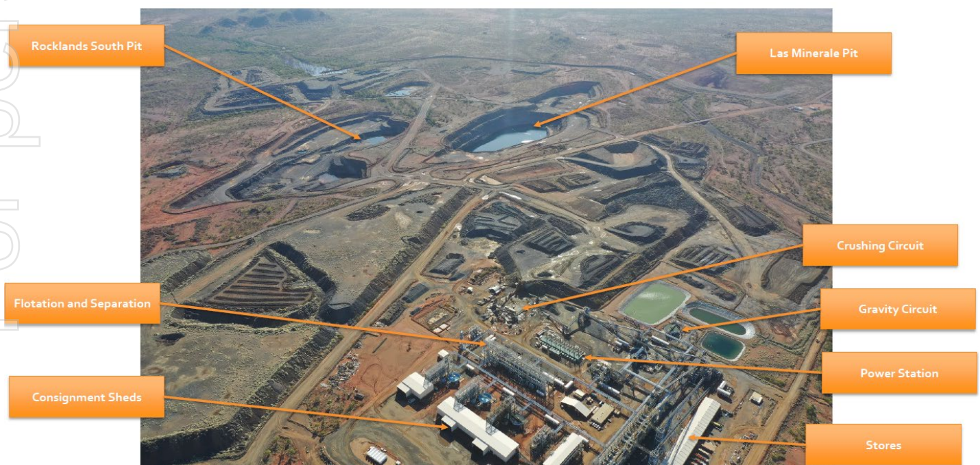
Figure 2: Facility-scale layout of Rocklands Processing Facilities.
