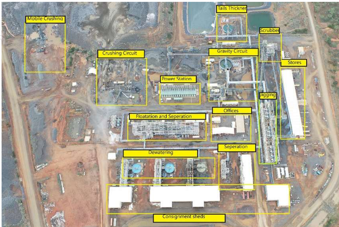
Figure 7-2. Rocklands processing plant configuration as at 2022.
