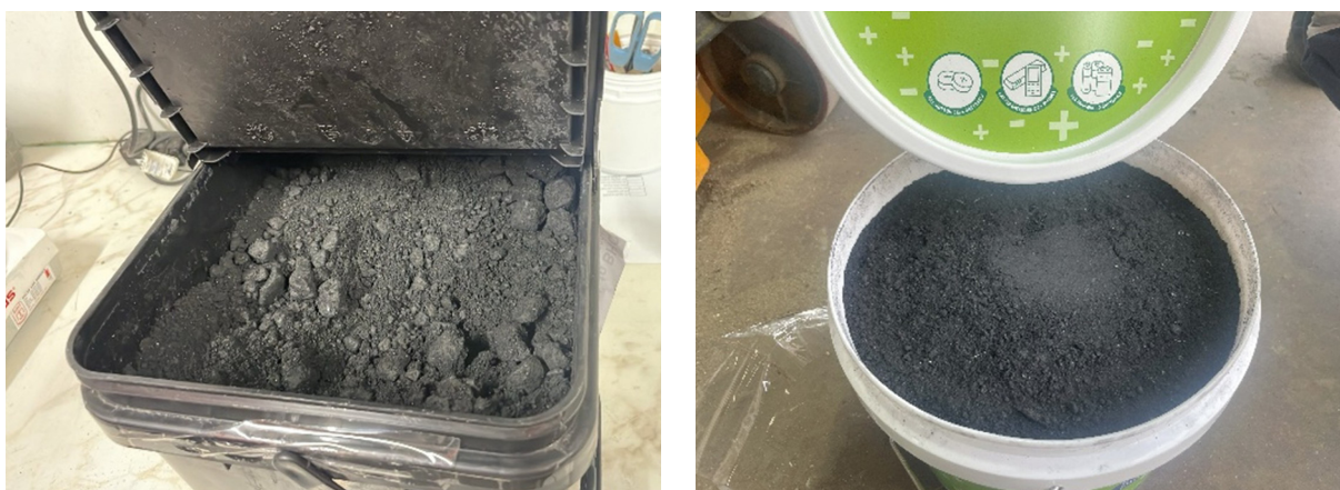
Figure 3 - Black mass samples from two separate sources processed at the BHTC.
