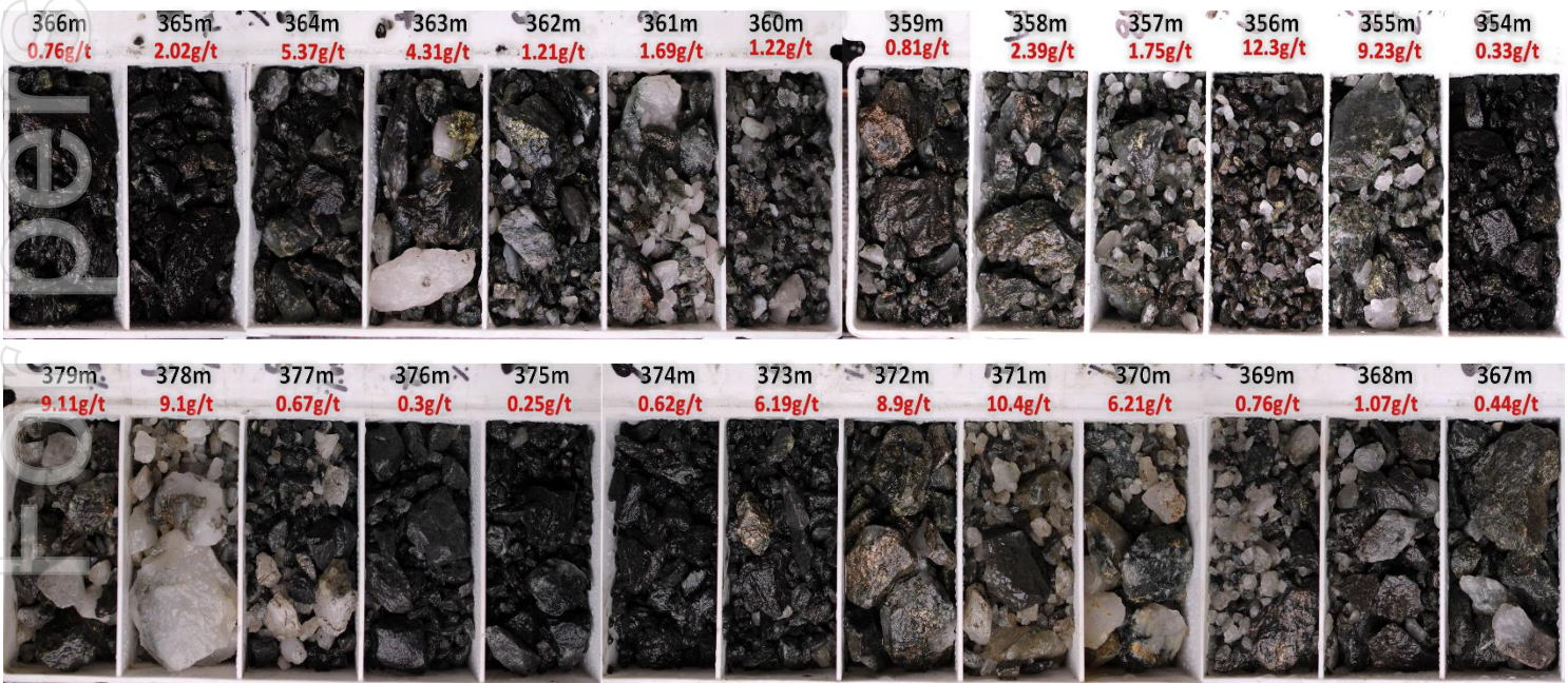
Figure 2 RC drill chips, hole 25PRC197, abundant pyrrhotite, chlorite alteration, sulphides and quartz carbonate veins including 10m @ 4.7 g/t from 355m.
