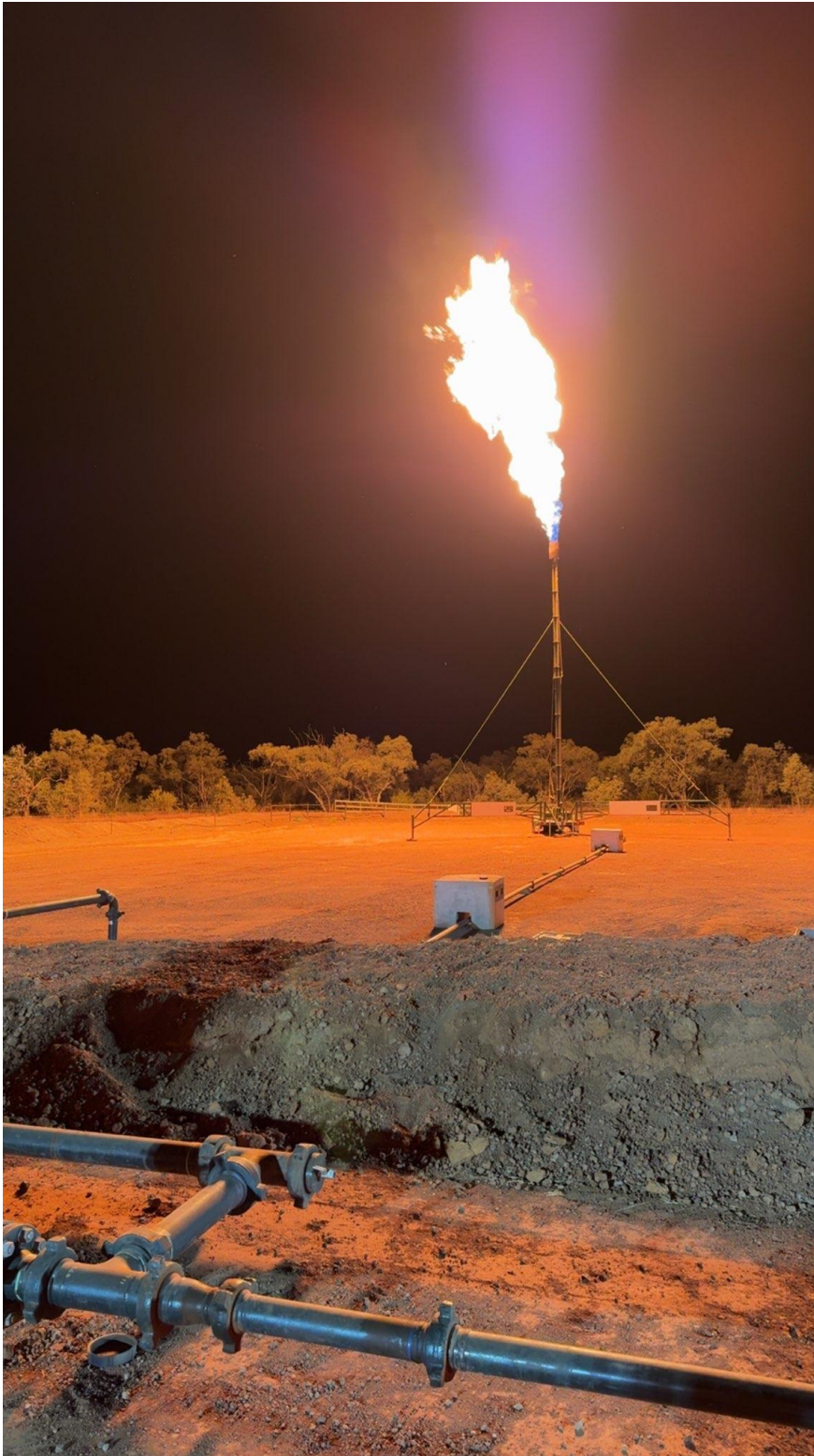
Carpentaria-5H gas flare during clean-up
