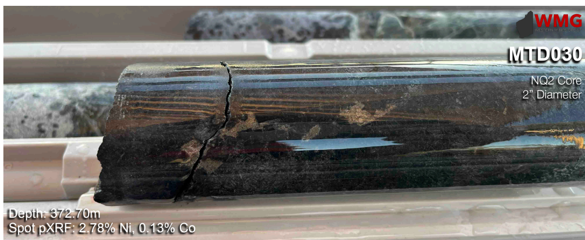
Figure 3: Photo showing examples of sulphide blebs and veinlets in hole MTD030 (EIS8)
