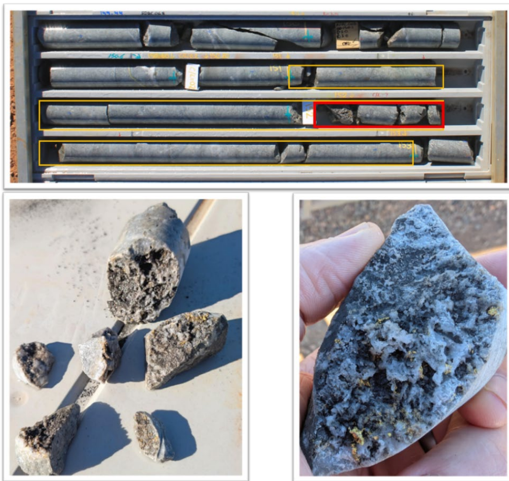
Figure 24: [TOP] shows the core from RDRC068, 149.44m to 153.13m, the yellow box highlights the interval 2m @116.3g/t from 151m to 153 m. The red box highlights the interval 0.2m @ 1,148 g/t Au from 152m-152.2m. [BOTTOM_LEFT] shows some core pieces from 152m-152.2m. [BOTTOM_RIGHT] shows a close-up of one of the pieces of core from the Bottom-Left figure with visible gold.
