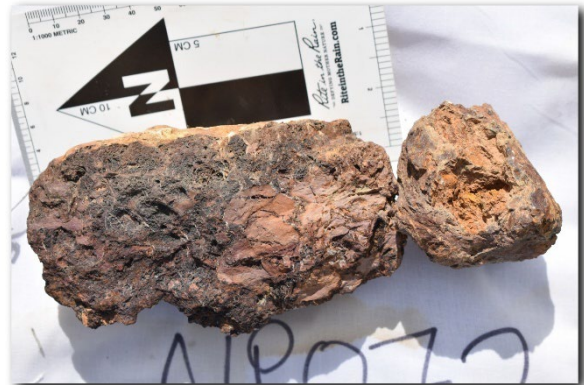
Sulphidic breccia, perhaps indicating the presence of a nearby “hot” intrusion, NP072. 0.11g/t Au, 1.13ppm Ag, 387ppm As, 299ppm Cu, 79.3ppm Sb and 1,050ppm Zn.
