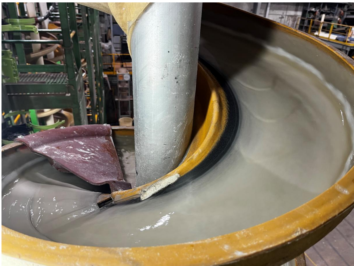
Figure 1: Spiral Separation stage of bulk metallurgical testwork from the Northern Silica Project.
