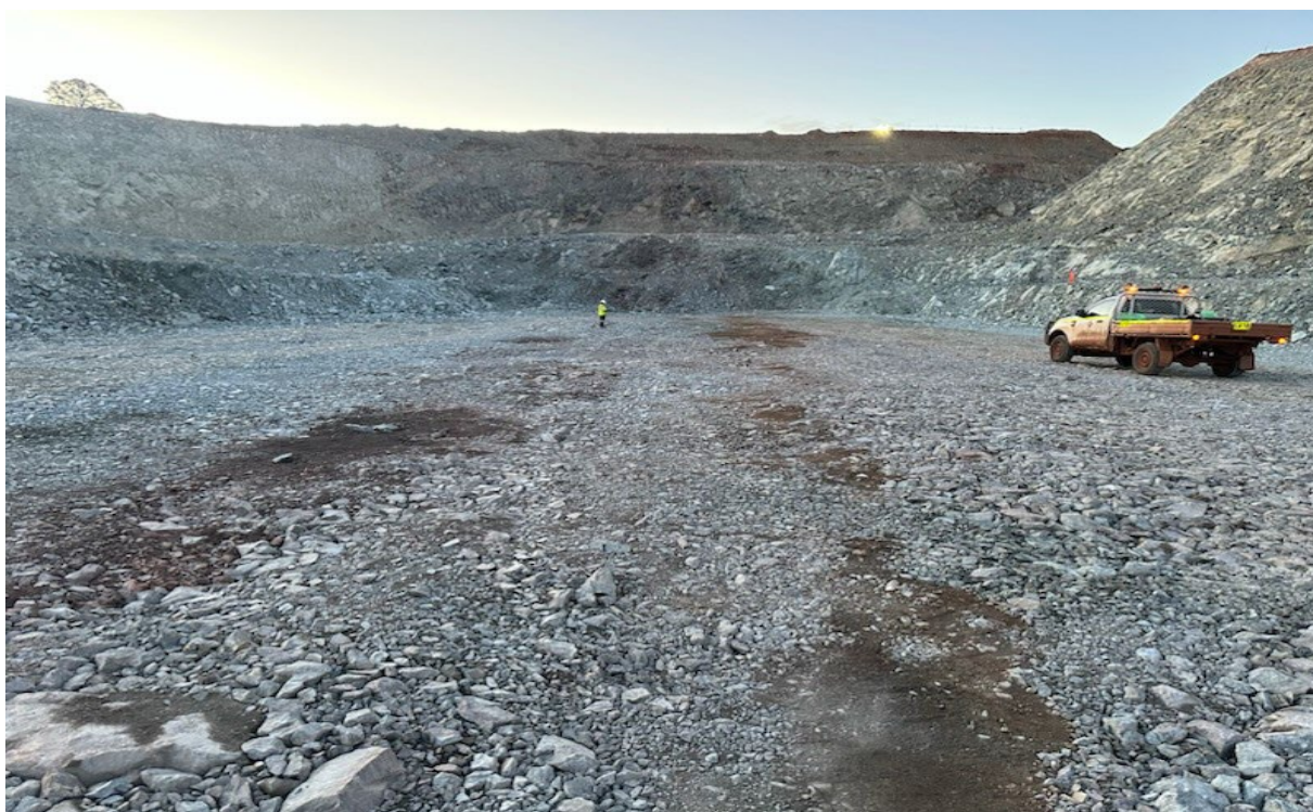
Devon Pit Gold Mine showing parallel lode structures (brown zones – photo taken 7 September 2025)
