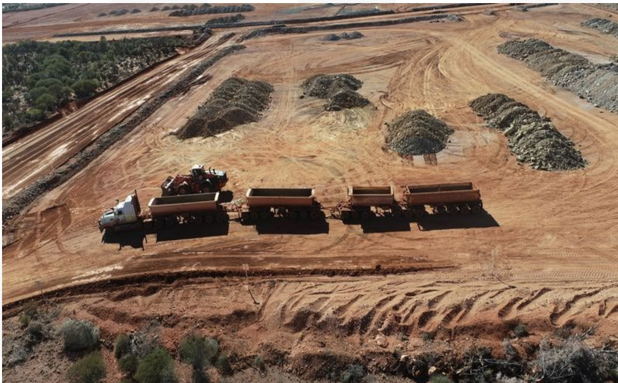
Loading a 4 trailer road train (quad) of approx. 100t at the Devon Pit Gold Mine (7 August 2025)
