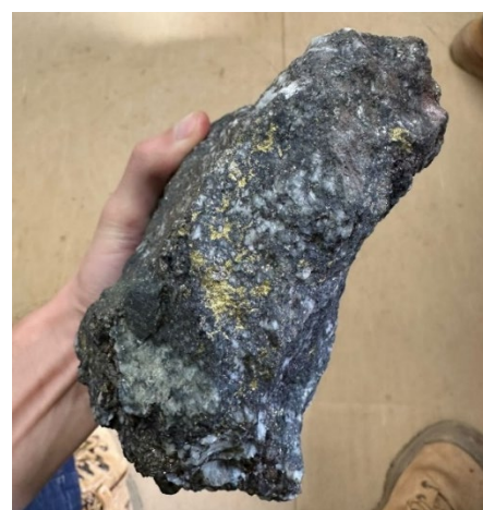
Hand specimen of ore showing visible gold 2 from the Devon Pit Gold Mine (photo – 6 September 2025)
