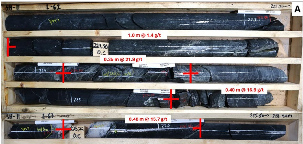
Figure 7-14: Example of Storheden Mineralized Interval in DDH SH-11. Mineralized Interval Returned an Average Grade of 73 g/t Au Along a Core Length of 3.05 m (ETW 1.96 m)
