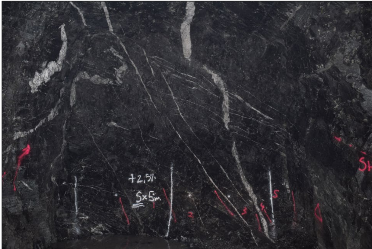
Figure 10-2: Underground Chip Sampling, Aurora Zone
