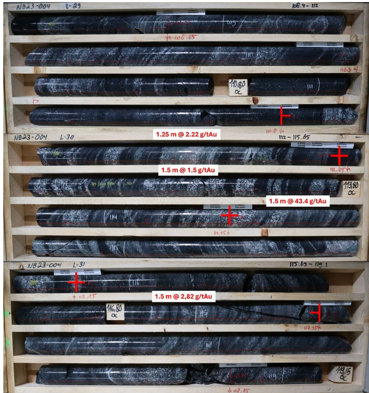
Figure 7-12: Example of Norrberget Mineralization in Drill Hole NB23-004. Combined Mineralized Interval Returned an Average Grade of 13.3 g/t Au Along a Core Length of 5.55 m (ETW: 5.22m)
