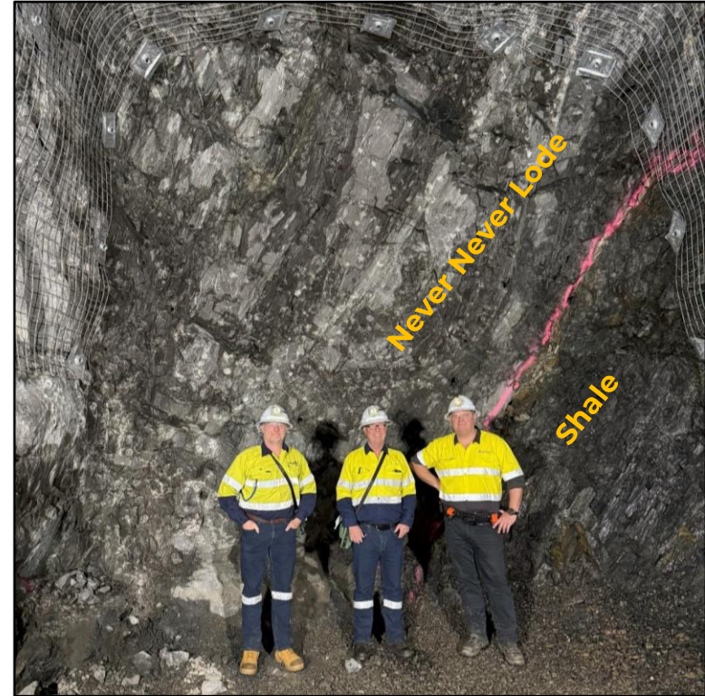
Tim Hewitt (COO), Mark Zeptner (CEO) and Simon Lawson (Deputy Chair) at the 235L Ore Drive South (2 August 2025). Pink spray line denotes contact between the Never Never lode and Footwall Shale units.
