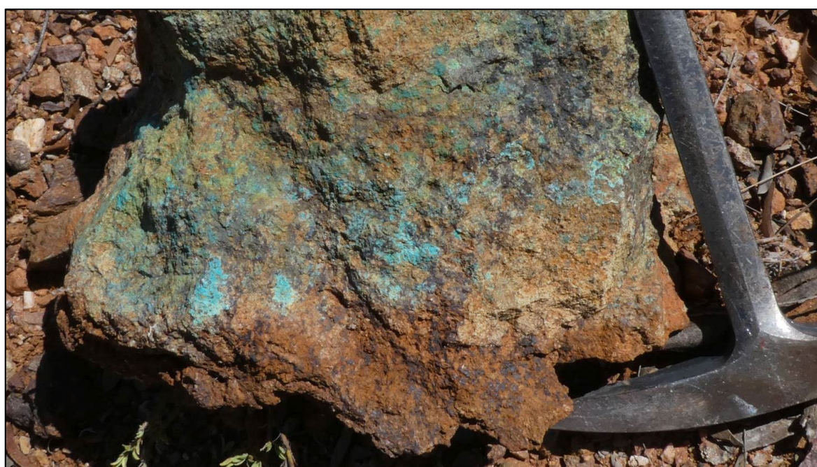
Figure 5. Sample NT0104 shows malachite staining on fractures within gossanous material, assayed 6.62% Cu, 0.10 g/t Au and 8 g/t Ag.
