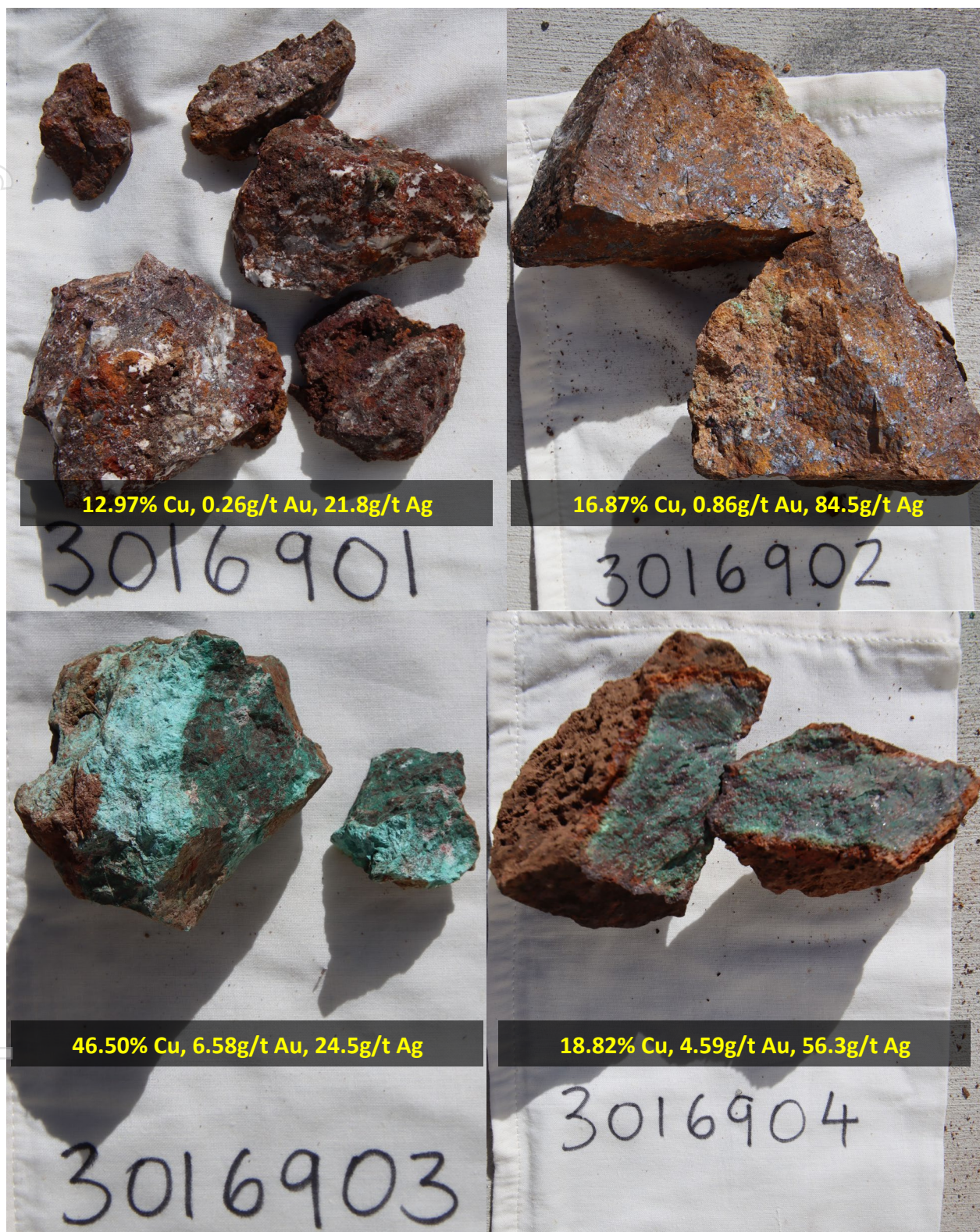
Figure 2. Recent mullock and rock chip samples collected from the Halls Reward Prospect. Descriptions are as follows: Sample 3016901 – copper oxide bearing ferruginous quartz, altered rock, iron oxide, native copper and malachite; Sample 3016902 – copper oxide bearing ferruginous quartz, altered rock, iron oxide, native copper, cuprite and malachite; Sample 3016903 – copper oxide bearing chrysocolla, malachite, ferruginous clay quartz and altered rock; and sample 3016904 – copper oxide bearing ferruginous siliceous gossan, iron oxide, malachite needles, cuprite, spongy silica, clay and altered rock.
