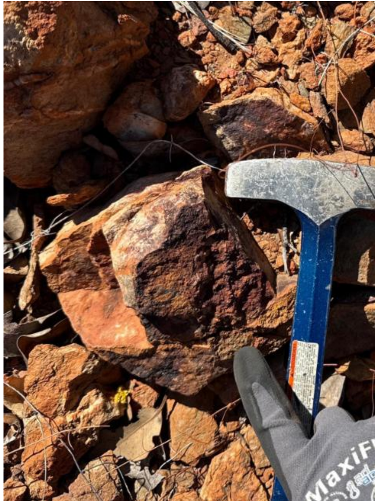
Figure 3. Sample MM2515: Quartz brecciated sandstone with hematitic-rare earth mineralisation assaying at 2.7% TREO, with 94% HREO and 13% DyTb.
