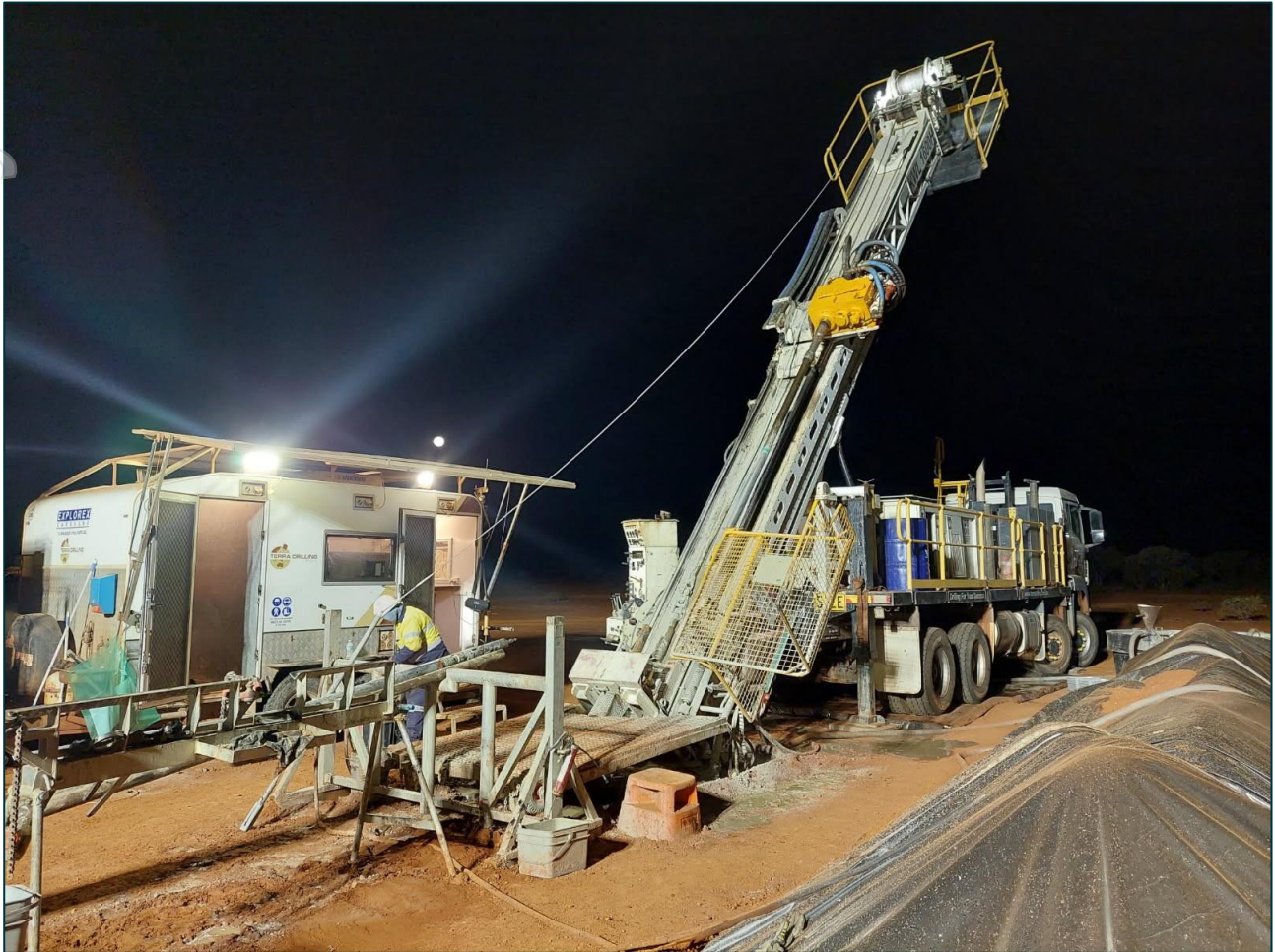
FIGURE 1: DIAMOND DRILLING IN PROGRESS AT IRONBARK
