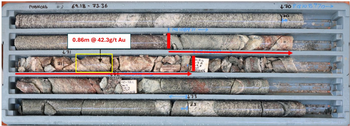
Figure 1: Posie Prospect drillhole PODH016 displaying quartz veining containing high grade gold: 0.86m @ 42.3g/t Au from 70.54m downhole depth . Core tray length is 1m with NQ2 sized diamond core from 69.2m to 73.4m downhole depth. Yellow box refers to the core presented in figures 2 and 3 below. Core processing and analytical laboratory methods are summarised in Appendix 3, Table 1 below.
