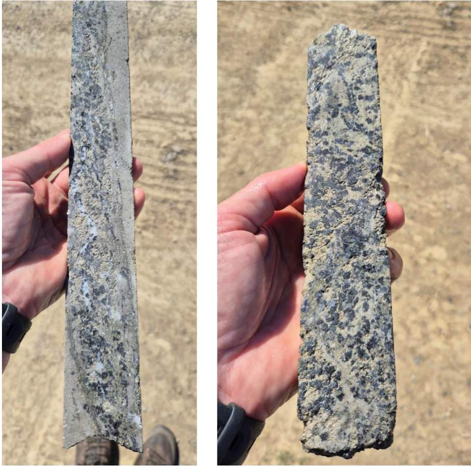
Figure 3: Photos from semi-massive sulphide zone comprising sphalerite, galena, pyrite and chalcopyrite with associated carbonate in ZRMDD064. Left – 340.55–340.98m, Right – 340.98–341.3m.
