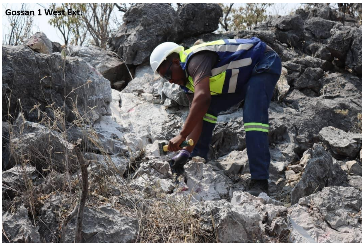
Image 1: Diamond saw channel cutting and sampling at the Gossan 1 West Ext. copper mineralised zone
