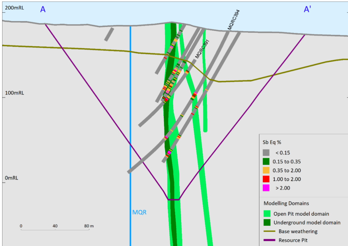
Figure 2 – A-A' section view facing east with open pit and underground domains illustrated with projected one metre downhole assays. Conceptual MQR open pit shell also projected onto section.
