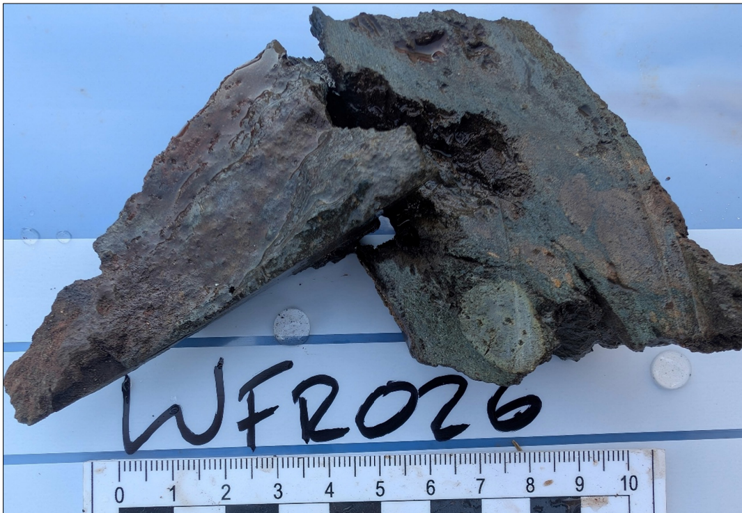
Photo 2. Rock sample WFR0026 returning 0.27g/t gold in float near soil anomaly at Olaf's Prospect. Dark green chloritic matrix with volcanic(?) clasts up to 5mm. Possible volcanic breccia.
