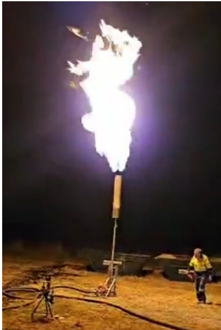
Figure 1: Production Test Well 271-KA03PT06 being choke tested
