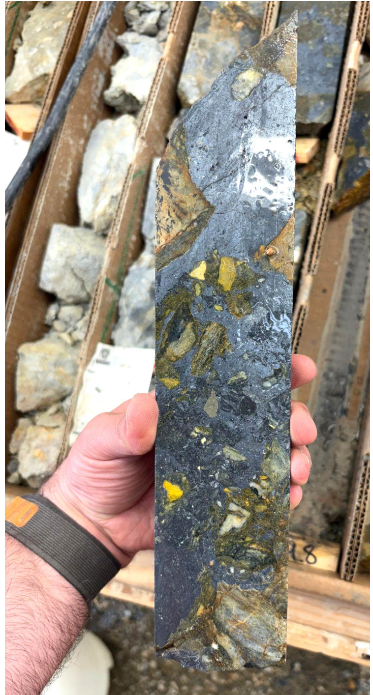
Fig 7. Typical “black breccia” in hole 25TCDC004, from 45.8 m. Metallic grey colour is massive stibnite breccia fill. HQ core, width of sample is 6.35cm. Part of sample 477214 from 45.46-46.3m that assayed 22.39% Sb.
