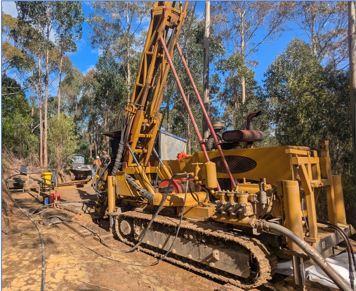
Figure 3 – Drill Rig Positioned over Diamond Drill Hole EVDD001
