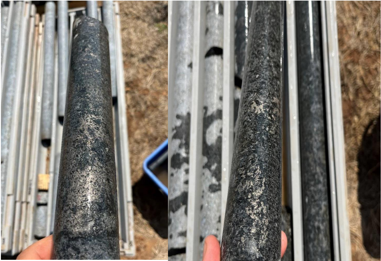
Figure 5. Photos showing examples disseminated and blebby sulphides in hole BRDD002. (Left) Nickel-Copper sulphides at 348m, (Right) Disseminated sulphides 338 – 342m Note core is NQ2 being 2 inches or 50mm in diameter
