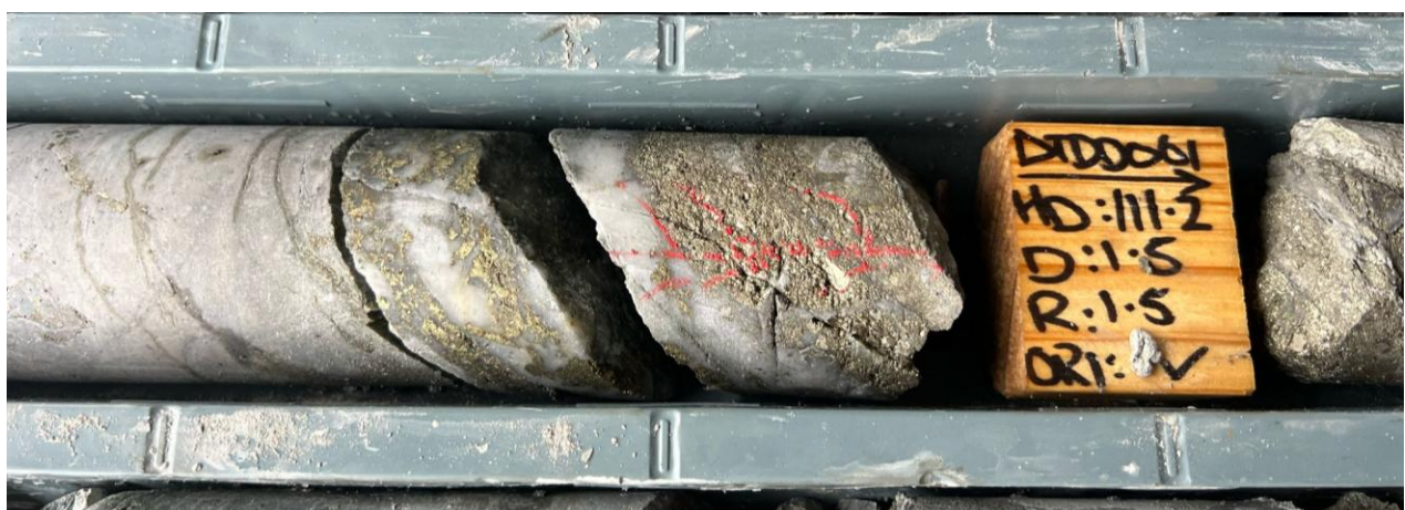
Figure 1. Intersection of the displaced Duffer Lode in DTDD061 – 100mm quartz-pyrite-chalcopyrite vein (110.9 – 111.25m)
