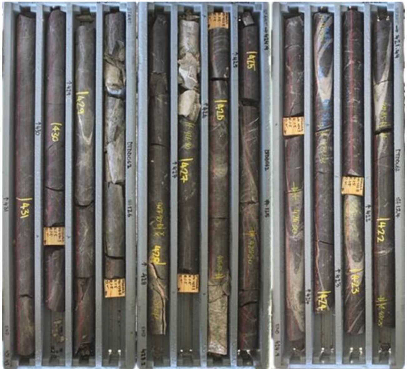
Figure 2. Intersection of potential down-dip extension of the displaced Duffer Lode in DTDD062, including pyrite +/- quartz veining up to 10mm with phyllic selvages (421.4 – 431.4m)
