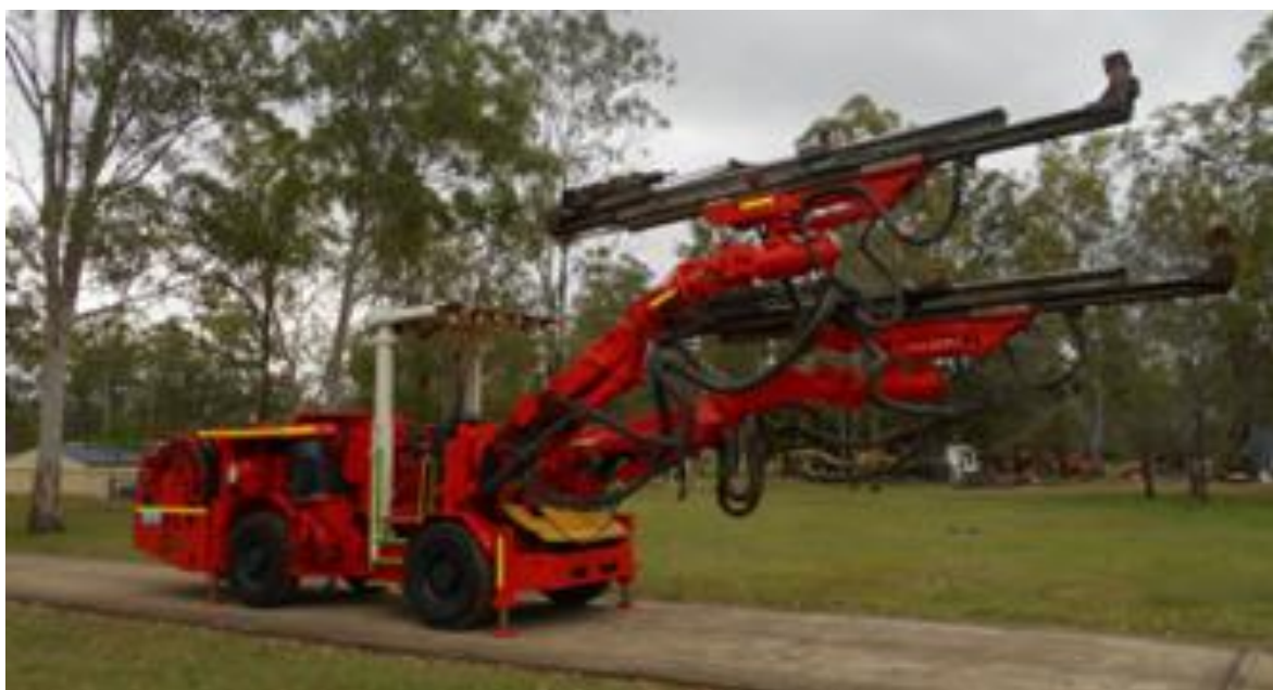
Figure 6. Twin-armed mechanical drill rig purchased for testing the Duffer Lode's interpreted southern extension.
