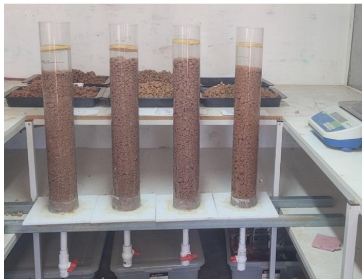
Figure 1: OZM inhouse Kappes percolation testwork columns
