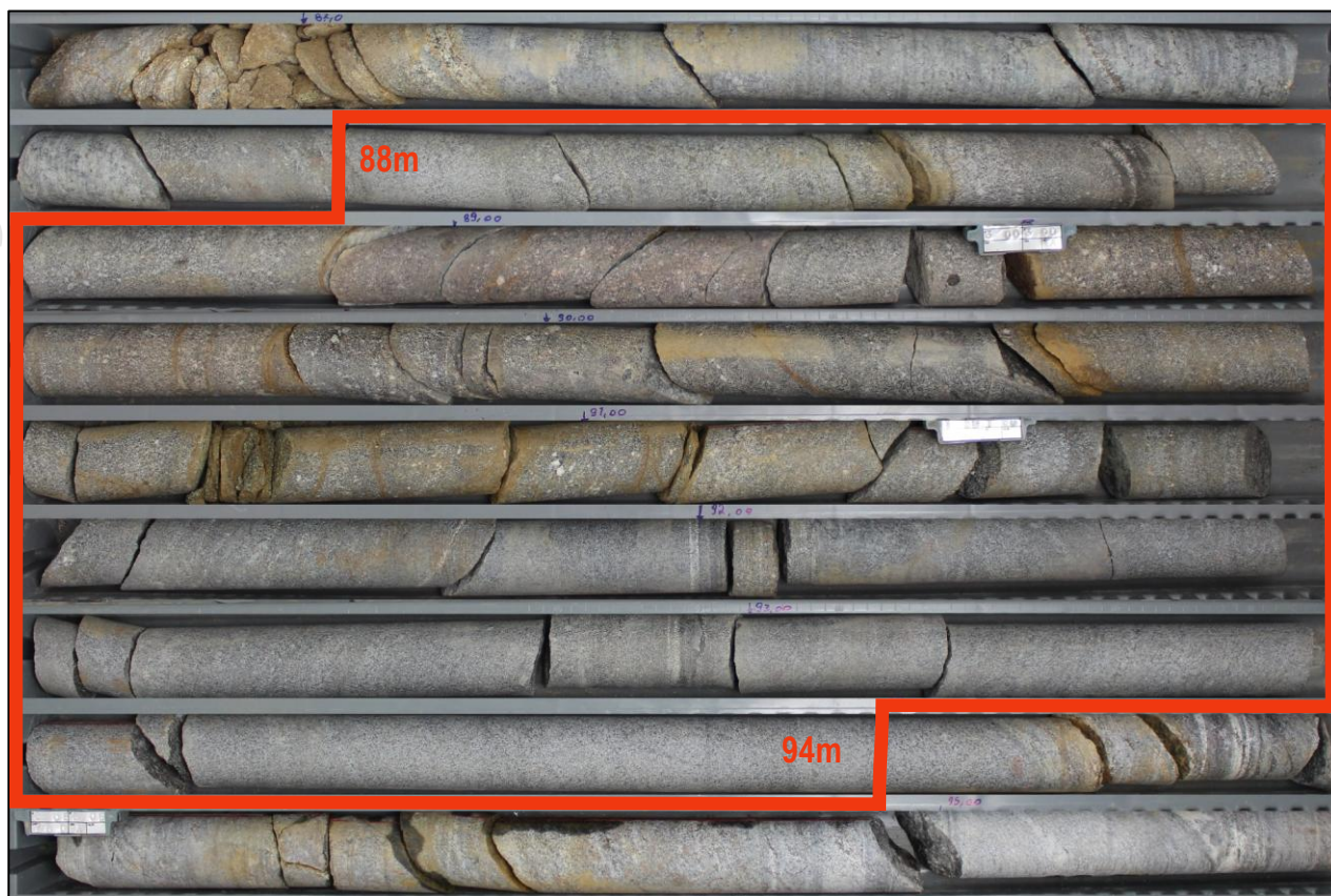
Figure 6: High-grade rare earth mineralisation in a monzodioritic melt: 6m averaging 3.1% TREO from 88 metres (JITDD0030)
