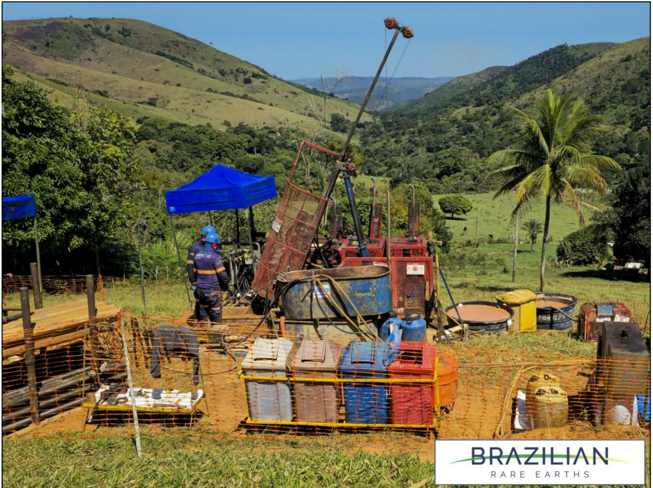
Figure 7: Diamond core drilling at Sulista East
