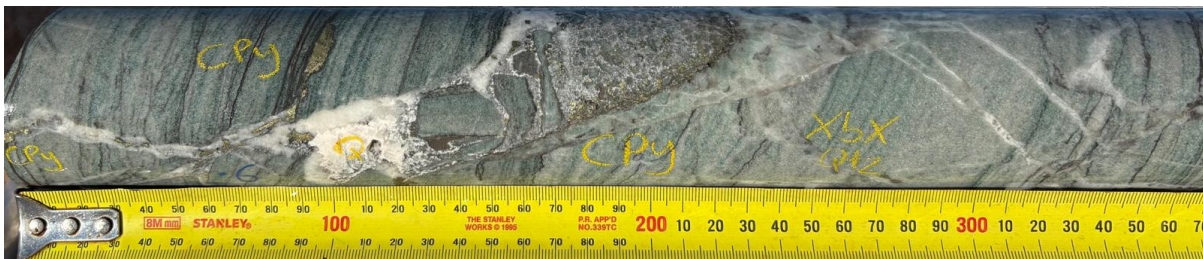
Figure 5 HQ core sample from 25IRC007D (from 438.6m) showing 2% chalcopyrite within a cross-cutting quartz-chalcopyrite filled breccia vein, in chlorite altered siltstone (*See Cautionary Statement)
