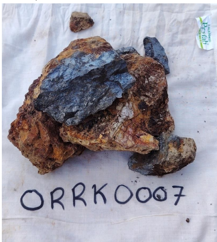
Figure 3 Orient South Rock Chip Sample ORK0007 ( 478.6 g/t Ag, 9.54% Pb and 5.18% Zn plus 0.27% Sn & 5.35% Sb )
