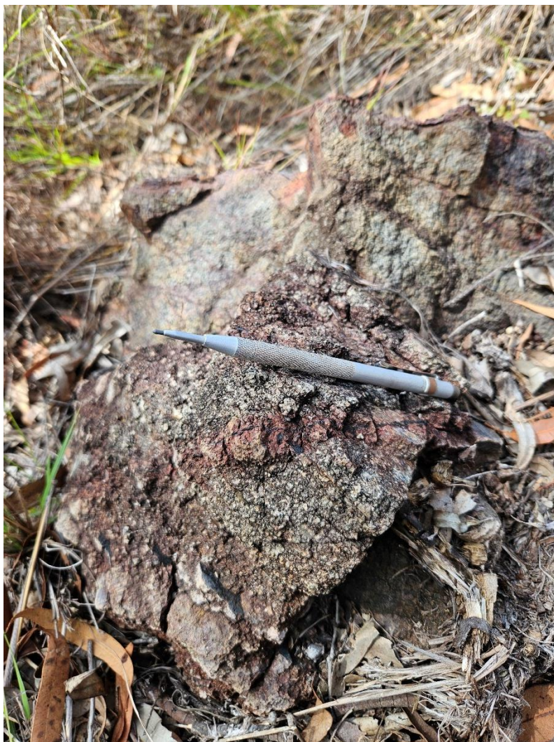
Massive rhyolite with ex-sulphide veins. Iron staining on the rim of the veins.
