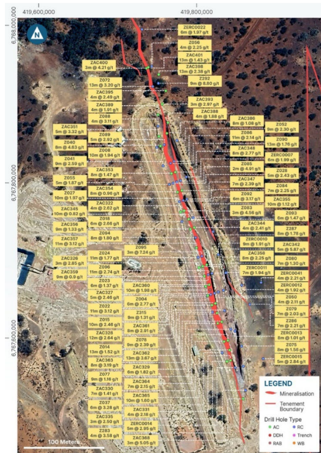
Figure 5: Aerial Photo of Zelica Trial Pit with Drilling and Projection of the Gold Mineralisation
